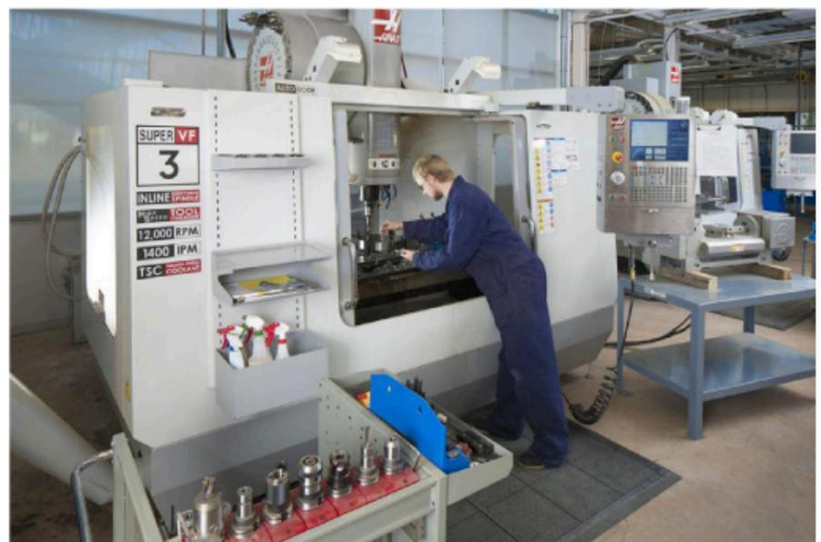
HAAS Super VF-3 vertical milling machine.
